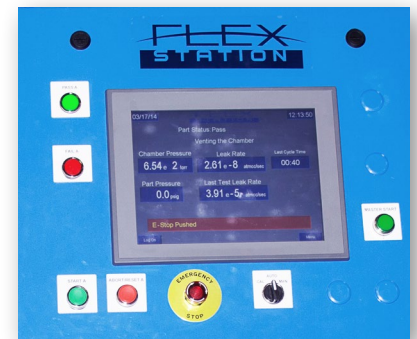
Industrial PLC with 10" color touch screen
