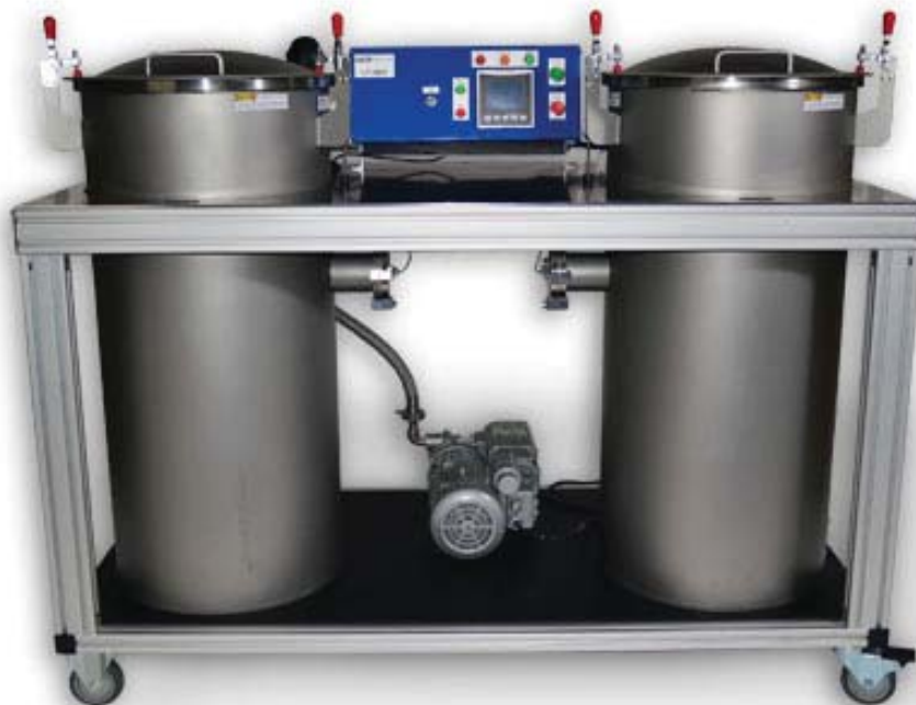
Body Armor Leak Testing Vacuum System
