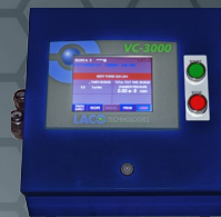
VC-3000 with PLC Automatic vacuum control
