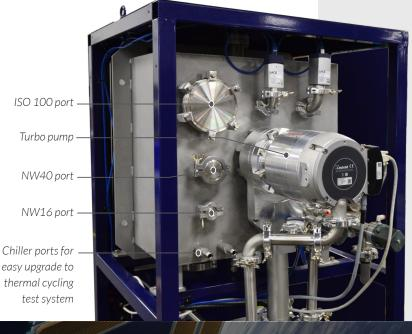
Programmable test recipes and data logging for vacuum,
