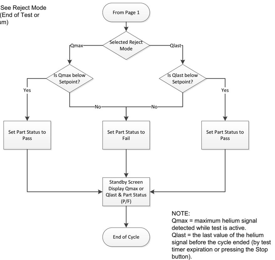
Fig. 13: Page 2 Auto Test Process Diagram
