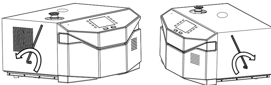
Fig. 20: How to remove the cover
