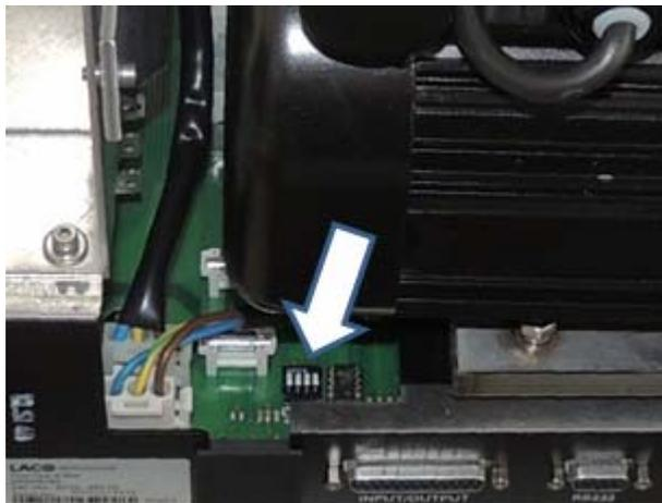
Fig. 47: RS485 DIP switches
