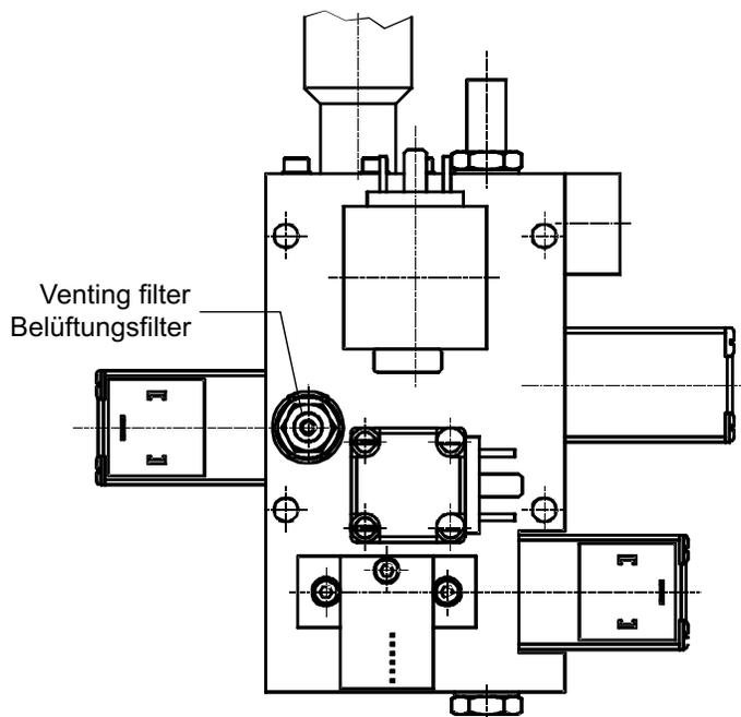
Fig. 24: Venting filter
