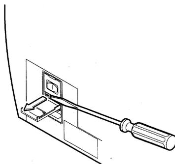
Fig. 28: Replace the mains fuses (2)
