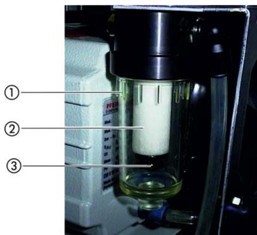
Fig. 18: Replacing the filter for the oil mist filter
