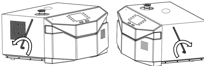
Fig. 16: How to remove the cover
