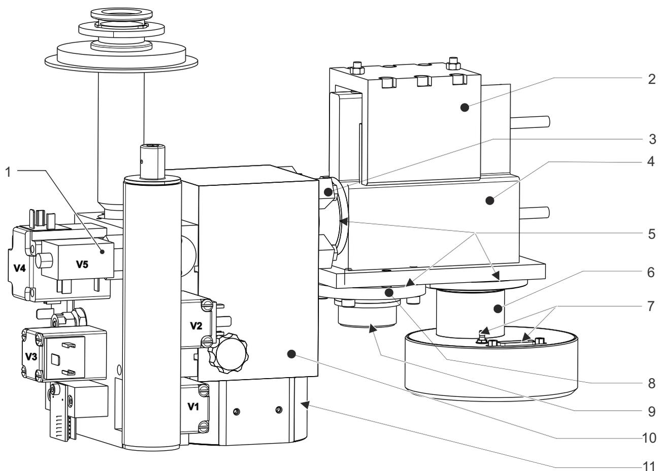
Fig. 38: TITANTEST™ Detection System complete
