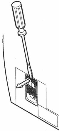
Fig. 27: Replace the mains fuses (1)
