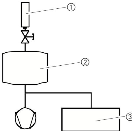
Fig. 14: Connection external calibration leak for partial flow.
