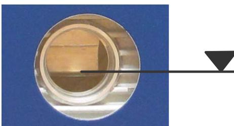
Fig. 17: Oil sight glass on the back of TitanTest™
