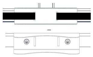
→ Attach rubber bumpers to base of cart using 2x lock washers and 2x M6 nuts.
