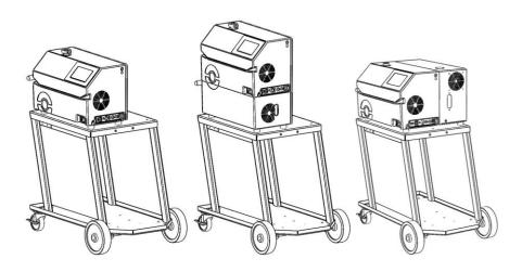
Mounting position for Compact or Tower configurations.
