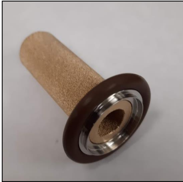
Figure 2: Bronze Filter Installation
