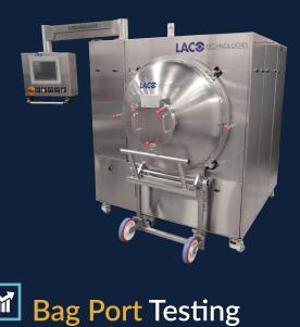
Single-use bags are not only susceptible to leaks in the bag itself but also the port seals. We have developed automated leak test systems just for port
