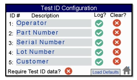
Up to 5 user defined Test ID data points can be configured on the Test ID Configuration screen. Descriptions can be entered on the touchscreen, or the user can load Default Test ID's by pressing the "Load Defaults" button. Select the "Log" icon if you want to log the data. Select "Clear" if you want the controller to delete the Test ID at the end of a completed test.
