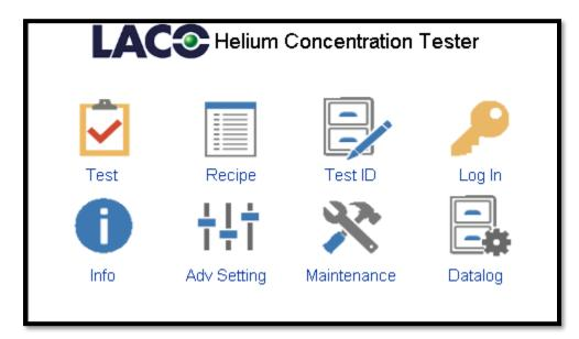
The home screen allows access to all LHCT controller software features. Press the desired icon to access the needed menu. The Home screen is accessible from any screen by pressing the home icon in the lower right-hand corner of the screen.
