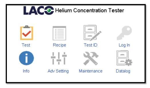
From the home screen one can access the Test, Parameters, Info and Advanced Settings screens. The home screen is accessible from any screen by pressing the home icon in the lower right corner. The Advanced Settings Menu screen is password protected by the password 1234.
