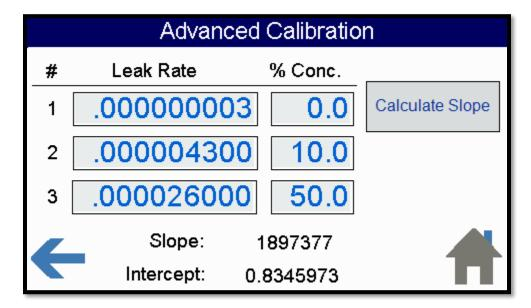
LACO performs a multi-point calibration on the tester based on the customer's typical helium concentration range. However, the user may likely need to perform an advanced calibration in certain cases such as leak detector, test condition or test environment changes.
