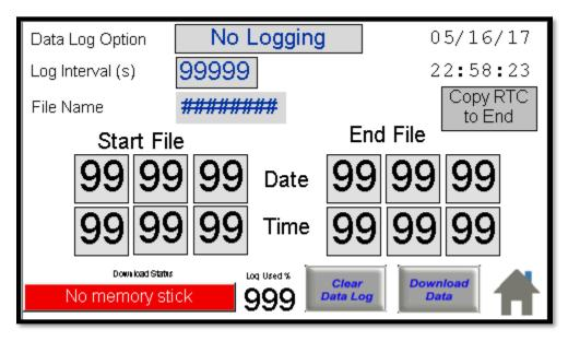
LHCT controllers can log process data to the controller and this data can then be uploaded with a connected USB disk drive (DOK). Users can log data by one of the following 3 data log methods:
