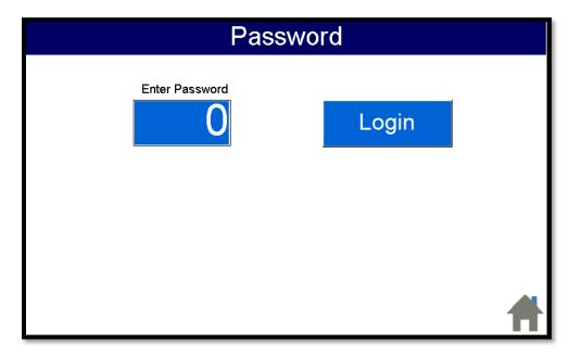
The above screen appears by pressing the Log In key icon. Enter the password for desired level of access. There are three access levels on the LHCT controller.
