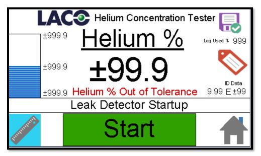
The test screen above loads upon system startup or can be accessed from the home screen by pressing the test screen icon. The following system states listed below are possible. When the system is powered on and the leak detector is not yet in the measure state then the Leak Detector Startup state will be displayed.
