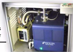
Inficon Mass Spectrometer
